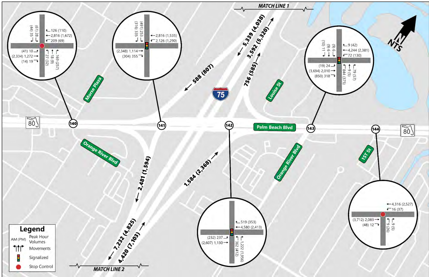
Figure 3.18 Design Year (2045) No Build DDHVs and Peak-Hour Volumes – I-75/Palm Beach Boulevard Interchange
